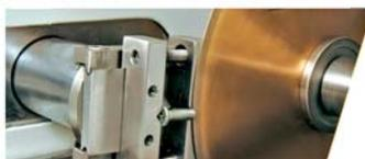
Various specimen vises can be mounted on dovetail plate
