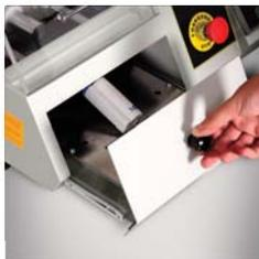
Recirculating coolant tank with 4,5 lt capacity
