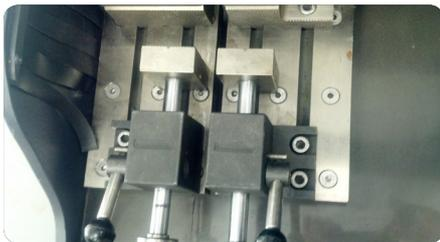
Twin T-Slotted clamping table with left & right Cam Vise
